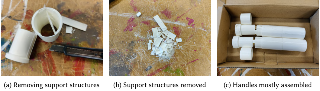
Fig. 11. The support structures need to be removed from the 3D printed parts.
