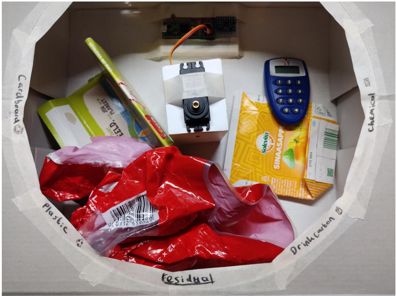
Figure 4: Bin with lid removed, all waste materials inside, motor and electronics visible.
